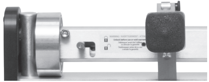
CAM LOCK IN LOCKED POSITION
