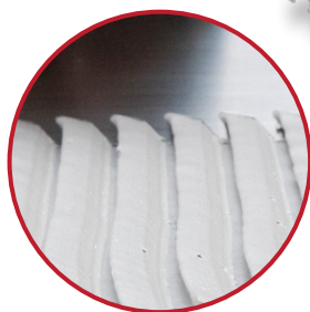
Overlapping and collapsible thinset action
