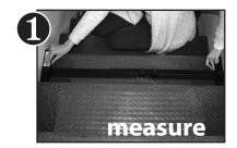
Place Stair Step Scribe 2<sup>™</sup> on stair tread, with pointed ends of guides facing the riser. Loosen all four knobs and extend the Stair Step Scribe 2<sup>™</sup>. Press the guides firmly against the edges of the step with the points touching the riser, then tighten all four knobs.
