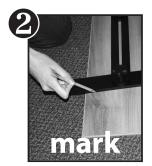
Lift the Stair Step Scribe 2<sup>™</sup> off the step and set it on the board to be cut. Align the points of the guides with one edge of the board. Holding the Stair Step Scribe 2<sup>™</sup> firmly in place, draw a line on each end of the Stair Step Scribe 2<sup>™</sup> along the sides of the guides.
