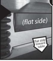
• Using the 4mm Hex Wrench, tighten the M8 Set Screws, starting with the center Screw.
