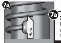
**THE ANVIL MAY BE USED AS A LOWER BLADE.** This can improve the cut quality on some softer products. Remove **Blade Stop** and place **Anvil** as shown (7a). Note: shorter screws (**M6** x **12** BH) are needed to do this. **See your dealer or contact Bullet Tools.**
