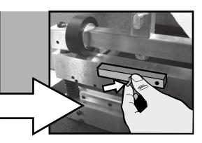
DO NOT LOOSEN, REMOVE OR ADJUST THE LENGTH of the M12 x 35 BH Retainer Screws - dealer repair only. Any adjustments to these bolt settings will VOID MANUFACTURER'S WARRANTY
