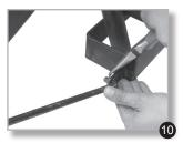
11. CAUTION: Do Not Pinch Fingers between agitator and melter. Lift lid of the melter and then angle agitator to fit into the melter with the long end of agitator on the same side as the shoe and thermometer.
