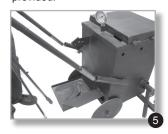
Connect two rods that were shipped inside of the melter to the levers on the melter handle.
