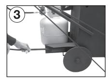
Keep applicator at least six feet away from combustible material. Remove product to be applied from the box and load it into kettle. If product has a plastic bag it will melt into heated product when stirred.
