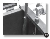
Connect torch to propane bottle and place torch into slot under melter.
