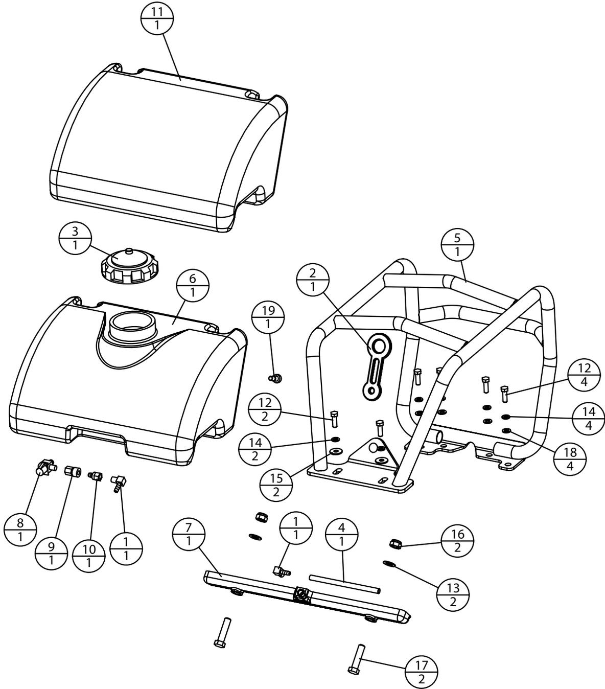
**PC3000, PC3000T ROLL CAGE/WATER TANK ASSEMBLY**
