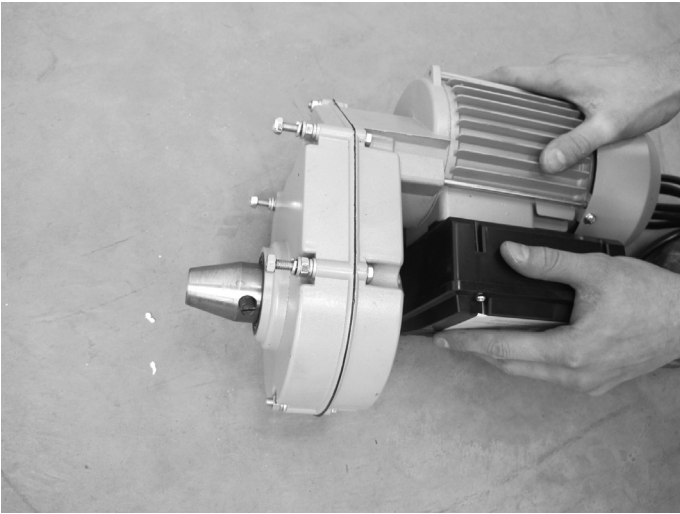
Remove nuts and washers from motor studs.
