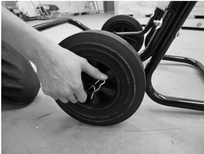
Insert wheel and fasten with cotter pin. (Hardware 3)
