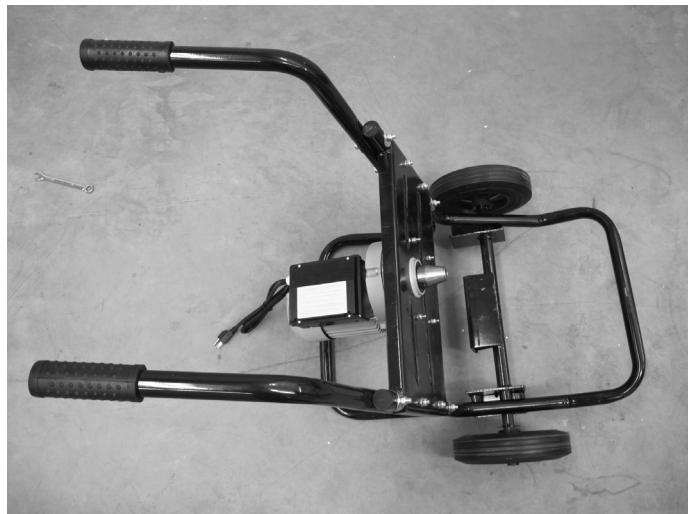
Finished frame with motor.
