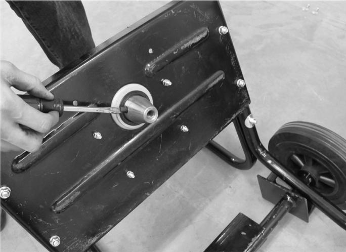
Align set screw using a standard screwdriver, perpendicular to mixer frame. **See Inset A**
