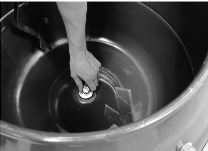
Two washers placed on bottom of drum, secured with bolt.
