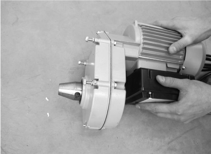
Remove nuts and washers from motor studs.
