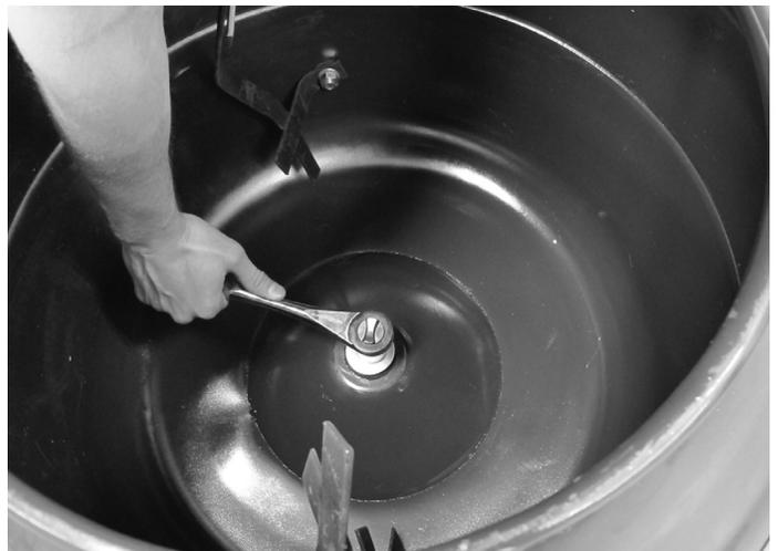
Use a 22mm socket to tighten drum to motor spindle.
