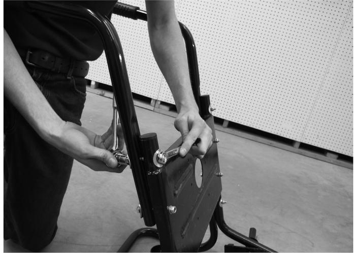
Fasten using a 14mm wrench and 14mm socket.
