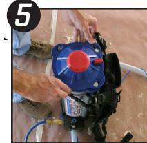
5 Place top cap back onto the tank. Once the top cap is securely in place, push down the lock release to ensure a tight fit.
