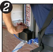
For a more thorough cleaning, empty all left over mud by opening the mud flow control to the highest setting and spraying the material into a bucket.
