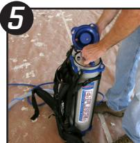
5 Remove piston by squeezing the gun trigger and pulling upward on the handle.
