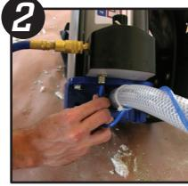
2 Insert the coiled blue air hose into the push-lock fitting in the bottom of the pneumatic assembly cover until it locks in place.
