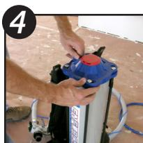
4 To remove the top cap, begin by loosening the top bolts 1-2 turns. Next, while holding the red lock release up, turn the top cap counter clockwise until it stops. Lift up on the cap to remove.
