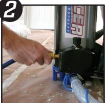
Connect the air compressor hose to the male air inlet on the pneumatic assembly. Set the air compressor to 40 psi and adjust as desired. DO NOT EXCEED 120 PSI.
