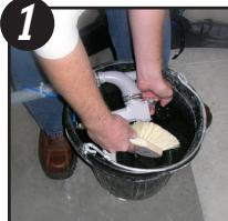
After every use the orifice of the gun should be cleaned. For best results, separate the gun and orifice plate and flush each with clean water.
