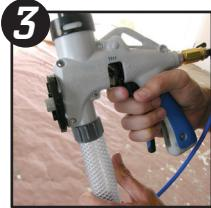
3 Attach mud hose assembly to the bottom inlet of gun. Tighten by hand. DO NOT OVER TIGHTEN.
