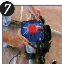
7 Place top cap back onto the tank by positioning over the top bolts and twisting clockwise. Once the top cap is securely in place, push down the lock release to ensure a tight fit. Tighten top bolts as necessary.
