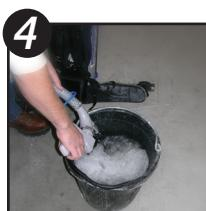
Replace the piston and lid and spray the clean water through. Repeat steps 3 and 4 until the sprayed water is clear.
