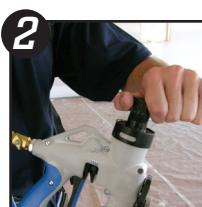
2 Next, remove the cap on the top of the gun port plug by turning counter clockwise. Prime the pump until the fill hose has filled with mud. **Failure to do this step will force air into the tank which will result in inconsistent textures.**
