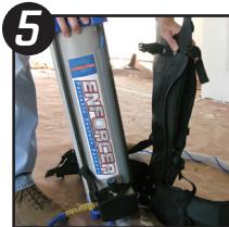
5 Place bottom of tank over backpack support bar and lock straps. Ensure the pneumatic assembly faces the right side. Tighten straps until there is a secure fit.
