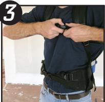
Once the air compressor hose is connected, put the backpack on. There are several adjustments that can be made to the straps to ensure a comfortable, snug fit. Once the backpack is in a secure and comfortable position, flip the fill/spray toggle switch to SPRAY and adjust the gun airflow by opening the ball valve at the base of the gun.
