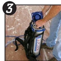
3 Remove piston by squeezing the gun trigger and pulling upward on the piston handle.
