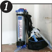
1 Remove the tank from your back and place on a secure, level surface.
