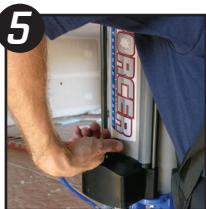
Once the desired mud flow is achieved, lock the mud flow control by pushing the outer portion of the dial back down. DO NOT ATTEMPT TO OVERTIGHTEN THE KNOB. DOING SO COULD RESULT IN COMPONENT FAILURE AND SERIOUS INJURY.
