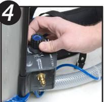
While holding down the trigger of the gun, begin adjusting the mud flow. Simply lift and turn the mud flow control in a clockwise direction to increase flow and turn counterclockwise to decrease flow.
