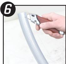
6 Cut one end of the fill hose  $\frac{1}{2}$ " deep lengthwise and connect this end of the fill hose to the outlet of your mud pump. Tighten clamp with screw driver.
