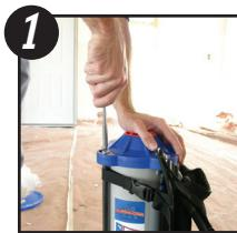
1 Flip toggle switch to FILL/OFF. To remove the top cap, begin by loosening the top bolts 1-2 turns.
