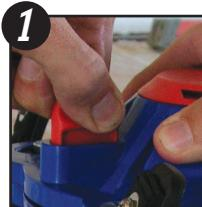
1 Flip the fill/spray toggle switch to the FILL position. Ensure all air pressure is released from the tank before filling is started. You will know this is done when the air stops exhausting from the pneumatic assembly.
