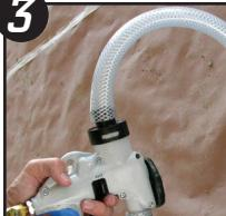
Place the end of the fill hose over the fill fitting on the gun.
