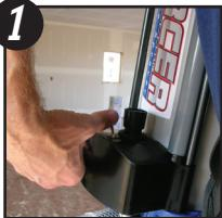
Ensure the fill/spray toggle switch is in the FILL/OFF position and that the mud flow control is turned all the way in the counterclockwise direction. Finally, make sure the air flow control on the gun is turned to the off position.
