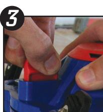
3 Pull upward on the red lock release to relieve the built up air pressure. Ensure all air pressure has been released before moving to the next step.
