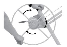
**2.** To raise the MARSHALLTOWN Drywall Lift rotate the winch wheel in the direction shown. The brake arm is spring loaded to hold the winch automatically at any height.
