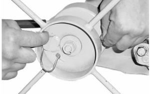
Loosen the cable from the mooring tab on the winch and pull it out from the winch drum. BE CAREFUL! A worn cable can have frayed strands. Wearing gloves will help protect your hands.
