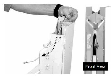
10. To reinstall the assembled telescoping sections, feed the crimped end of the cable through the frame sheave pocket from the top and over the top of the sheave as shown.
