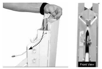
4. Feed the crimped end of the EXT48 cable through the frame sheave pocket from the top. It is VERY IMPORTANT that the cable passes OVER THE TOP of the cable sheave as shown here.
