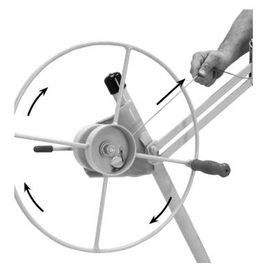
7. Feed the cable through the winch drum and secure it firmly behind the mooring tab as shown. Rotate the winch wheel in the direction indicated to take up the slack in the cable.
