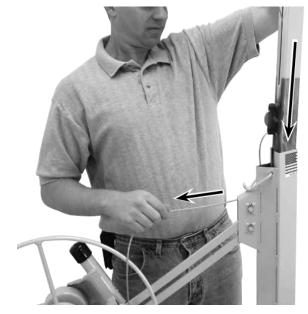
6. Pull the slack cable through the sheave pocket and slide the telescoping sections into the frame housing.
