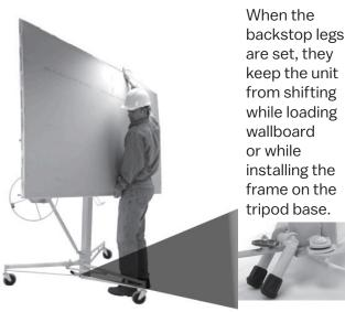
**1.** To Load: Set the backstop on the tripod base to hold the unit in position. Extend the cradle outriggers to properly support the drywall, tilt the cradle, and swing out the cross arm support hooks. Load the MARSHALLTOWN Drywall Lift from the front as shown with the face paper of the drywall contacting the cradle.
