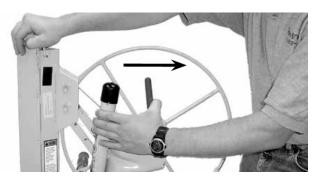
**5.** Place your right hand on top of the frame and pull the winch assembly towards you. While pulling the winch towards you, grip the brake arm sufficiently to prevent back-lash of the cable on the winch.
