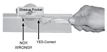
6a. Insert the crimped end of the cable into the sheave pocket at the end nearest the end of the "B" section as shown.
