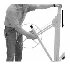
**6.** While holding the slide bar lock in this disengaged position with your right hand, push down on top of the telescoping section with your left hand. This action will cause the winch assembly to move toward the frame.
