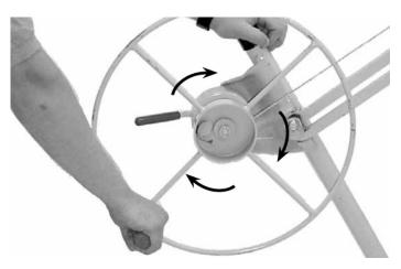
13. Rotate the winch in the direction shown to take the slack out of the cable.
