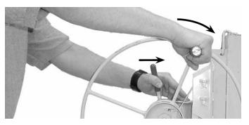
**3.** To move the winch into the working position rotate the winch forward slightly with your right hand while raising the brake arm with your left hand.
