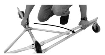
Begin by setting up the tripod base: press down on the slide yoke pin clip and swing the outer legs out until they lock in the working position (note the holes on the bottom of the slide tube).
