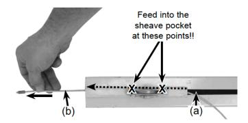
7. Feed the crimped end of the cable down into the slot (a) of the "B" section and out the bottom end of the telescoping section (b) as shown. Pull the cable completely through to remove the slack.
