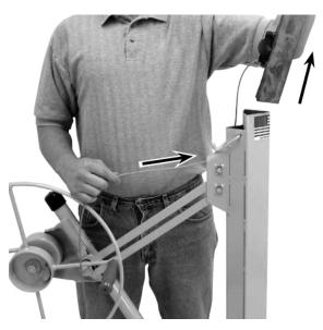
3. Remove the two telescoping sections completely from the frame housing. Pull the cable completely out from the frame along with them. Remove the "A" Section from the "B" Section as shown below. BE CAREFUL for loose strands or frays on the cable.
