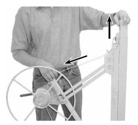
2. Pinch the two telescoping sections together and lift them out as a unit. Pulling the cable will help to raise them.
