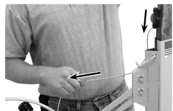
11. Pull the slack cable through the sheave pocket and slide the telescoping sections into the frame housing. As the telescoping sections lower into the frame, the slack cable will be drawn back up over the sheave.
