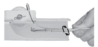
6b. With a clockwise motion like that of tightening a screw driver, twist the cable installation tool while holding the crimped end of the cable up into the sheave pocket. The cable will pop loose from the tool and pop up through the sheave pocket as shown in this cut away view.
