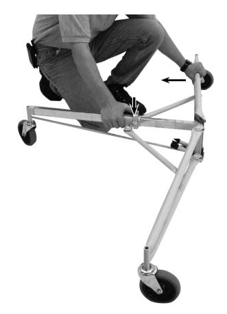
**10.** To collapse the tripod base, press down on the slide yoke pin clip and swing the legs in until they lock in the closed position.
