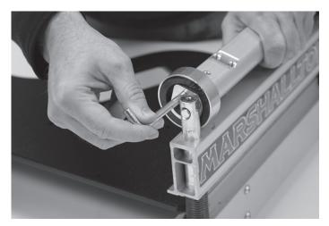
6. Rotate the Handle Base on the top of the Cutter Assembly (F) and insert the Locking Pin (G) into the side.
