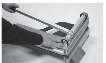
2. Place material to be cut on the table with the finished side up and slide past the blade to the desired length. Press flooring against the Bed Fence and hold firmly in place to ensure a clean and accurate cut. Press handle down until the blade touches the material and then firmly press down on the handle until the material is cut.
