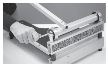
1. Press down handle and carefully remove the Cam Locking Pin. Carefully raise and release the handle.
