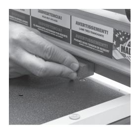
Beveled edge on blade facing retaining screws
