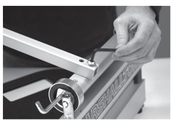
7. Attach Handle (D) to the Handle Base using Hardware Set (L).
