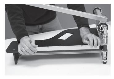
8. Place the Bed Fence (E) into the holes on the right side of the Bed (A).
