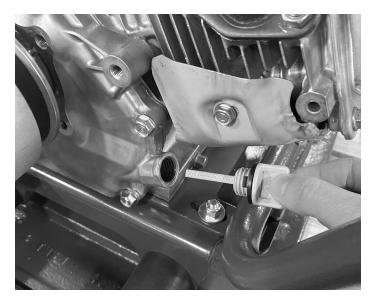
**5.** The plate compactor ships with engine oil, but check prior to starting.
