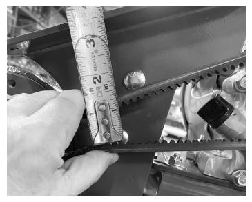
6. Correct belt tension can be checked by using moderate pressure to squeeze both sides of belt. Approximately 1" of movement is correct tension. Loosen engine mounting plate and adjust to correct belt tension. Retighten.
