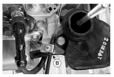
**4.** The throttle cable/lever comes connected to the handle (A) and carburetor (B). Move throttle lever and watch movement on the carburetor to insure correct operation.
