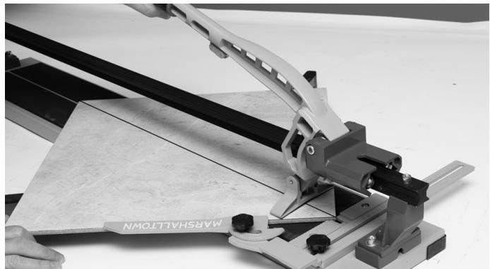
4. Apply increasing downward pressure on handle until the tile snaps.
