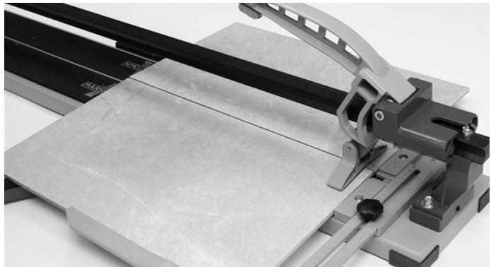
3. After scoring, and without moving the tile, position the handle so that the breaker foot is directly above the tile's front edge (at the stop).
