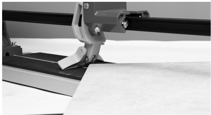
2. Carefully lower wheel until it makes contact with tile and then apply consistent pressure while scoring full length of the tile.
