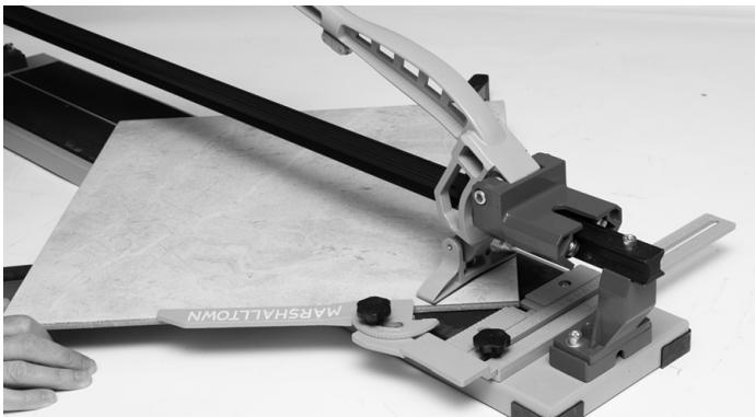
3. Flip the breaker down and position slightly away from the front edge of the tile.
