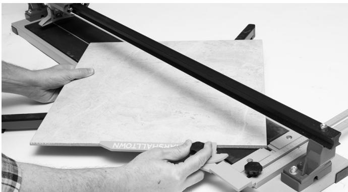
1. Adjust angle guide to desired angle and place the guide against the tile.
