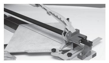
4. Apply increasing downward pressure on handle until the tile snaps.
