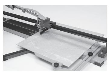
2. Place the cutting wheel on the rear edge of the tile and slide the wheel forward by pushing the handle down, scoring the tile as the handle is pushed forward. It is important to make this scoring cut in one continuous motion, scoring only once per tile.
