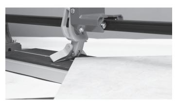
2. Carefully lower wheel until it makes contact with tile and then apply consistent pressure while scoring full length of the tile.
