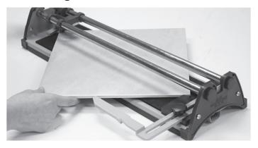
1. Adjust angle guide to desired angle and place the guide against the tile.
