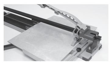
3. After scoring, and without moving the tile, position the handle so that the breaker foot is directly above the tiles front edge (at the stop).
